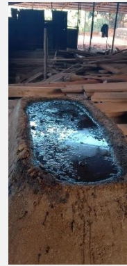
Gāre mortar prepared at Gokaṛṇa and left for fermentation
